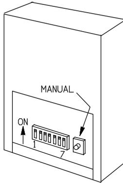
**Use Caution** when replacing access panel on DRN4. Excess pressure could change switch settings when you slide it closed.
